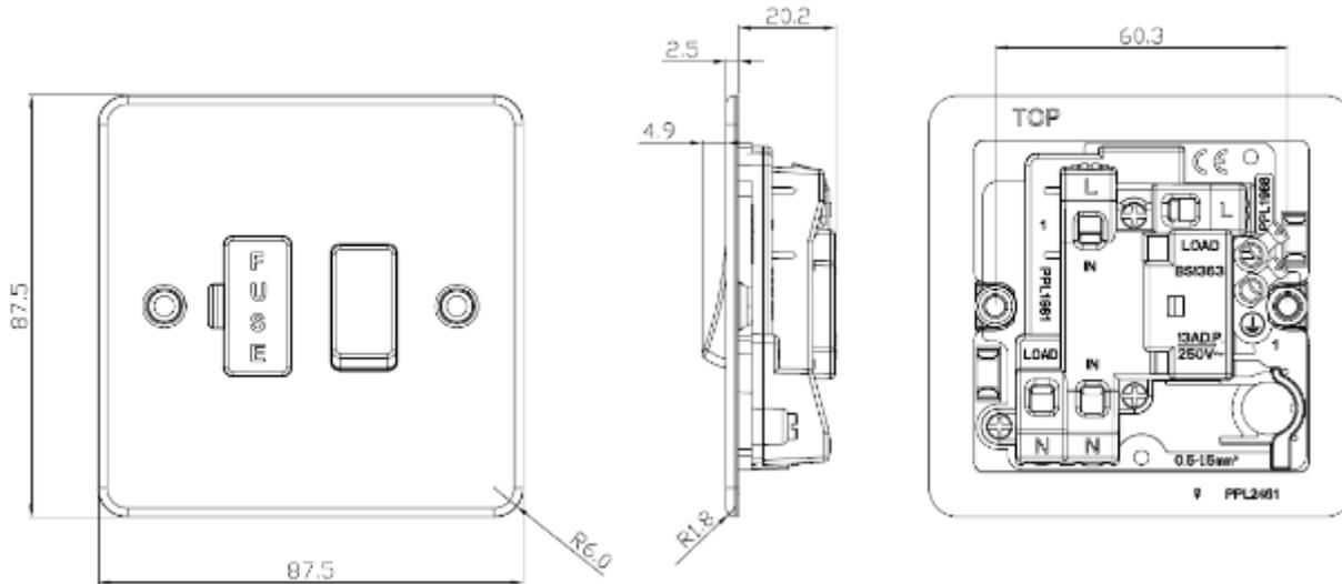
Fused spur units or connection units are an electrical switch with a built in fuse, designed for appliances that do not have or require a fused plug top. Fused spur units are also used for high powered electrical equipment with heavy continuous load, so that the appliance can be isolated by a single cable from a ring main for safety and maintenance purposes. 13A rated available with and without a double pole switch, neon and flex outlet.
