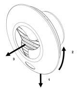
To refit the cover, reverse the above procedure. The iris shutter should be in closed position after refit. If not, wait approximately 1 min after fan switch off allowing the actuator to retract back in the closed position and then refit the cover adain.
